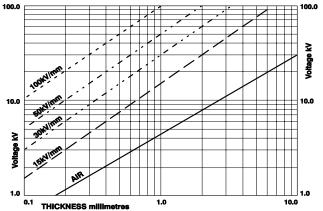
Breakdown voltage against thickness for materials of different dielectric strengths This graph is useful if you do not have a standard to work to and wish to know more about how to establish a test voltage.
